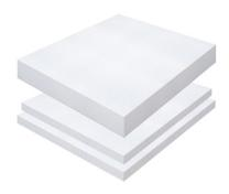
Insulation panels in moulded expanded polystyrene EPS, with CE marking compliant with Standard UNI EN 13163, with Thermal conductivity  $\lambda_{\scriptscriptstyle D}=0.033\,\text{W/mK}$  Standard EN 12667, Compressive strength  $\geq 200\,\text{kPa}$  Standard EN 826, compliant with Minimum Environmental Criteria (CAM - Criteri Ambientali Minimi)
