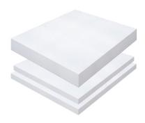
Insulation panels in moulded expanded polystyrene EPS, with CE marking compliant with Standard UNI EN 13163, with Thermal conductivity  $\lambda_{_{D}}=0.033\,\text{W/mK}$  Standard EN 12667, Compressive strength  $\geq 200\,$  kPa Standard EN 826.
