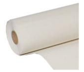
Synthetic membrane made from PVC-P, white coloured for its entire thickness, with high solar reflectance index (SRI). Reinforced with polyester mesh, produced by coextrusion or by coating, resistant to UV rays.
