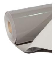
Synthetic membrane made from PVC-P, produced by coextrusion or coating, with signal layer, dimensionally stabilised with glass fibre, resistant to UV rays. Product with CE marking compliant with Standard EN 13956 and EN 13967.
