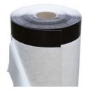
Synthetic membrane made from modified flexible polyolefin TPO, with single layer, obtained by coextrusion, resistant to UV rays, dimensionally stabilised with glass fibre and bonded on the bottom side to a self-adhesive, non-woven geotextile protected by a removable siliconised PE film.
