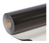
Synthetic membrane made from modified polyolefin TPO, with single layer, obtained by coextrusion, resistant to UV rays, reinforced with polyester mesh. Products with CE marking compliant with standard EN 13956.
