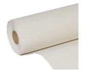
Synthetic membrane made from modified flexible polyolefin TPO, white coloured for its entire thickness, with high solar reflectance index (SRI). Obtained by coextrusion, resistant to UV rays, reinforced with polyester mesh. Products with CE marking compliant with standard EN 13956.
