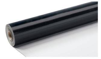
Synthetic membrane made of PVC-P by coextrusion dimensionally stabilized with glass veil, UV resistant.
