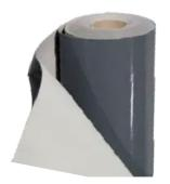
Synthetic PVC-P membrane reinforced with polyester mesh, equipped with signal layer, produced by co-extrusion, UV-resistant.
